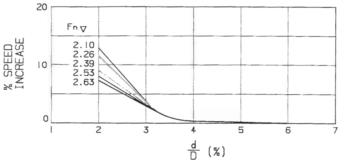
FIGURE 7. PROPELLER TIP CLEARANCE (SPEED INCREASE AT CONSTANT HORSEPOWER)
