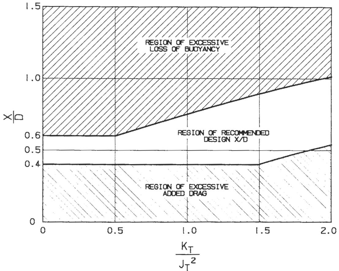
FIGURE 3. PROPELLER LOCATION IN TUNNEL
