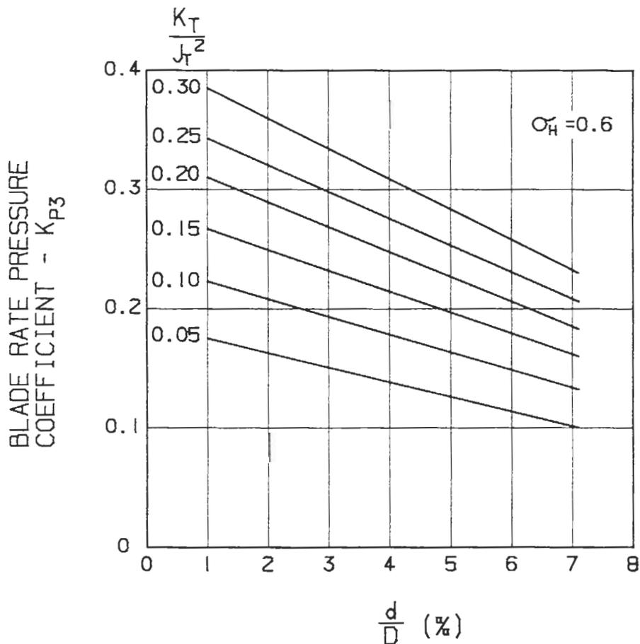
FIGURE 8. BLADE RATE PRESSURE COEFFICIENT FOR A PROPELLER WITH THREE BLADES
